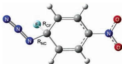
Figure 1. Bond length variables, R_{CF} and R_{NC} , in the S_NAr reaction between azide ion and 4-fluoronitrobenzene.
